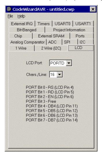
Using the **LCD Port** list box you can specify which port is used for connecting the alphanumeric LCD. The **Chars./Line** list box allows you to specify the number of characters per display line. This value is used by the **Icd\_init** function.
