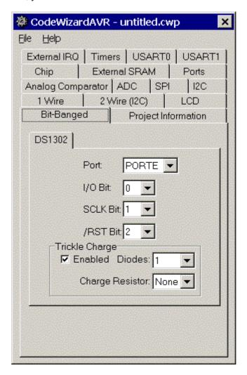
Using the **Port** list box you can specify which port is used for connecting with the DS1302. The **I/O Bit**, **SCLK Bit** and **/RST Bit** list boxes allow you to specify which port bits are used for this. The DS1302's trickle charge function can be activated by checking the **Trickle Charge|Enabled** check box.
