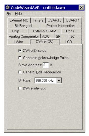
The AVR chip's 2 Wire interface can be enabled by checking the **2 Wire Enabled** check box. If the **Generate Acknowledge Pulse** check box is checked the ACK pulse on the 2 Wire bus is generated if one of the following conditions is met:
