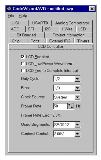
The ATmega169V/L on chip LCD controller can be enabled by checking the **LCD Enabled** check box. By checking the **LCD Low Power Waveform** check box, the low power waveform will be outputted on the LCD pins. This allows reducing the power consumption of the LCD.
